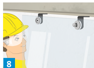
8 Verify perimeter gaps (a to f) and alignment of the glass panels, adjust as necessary.
