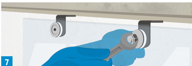
7 Holding the glass panel in place, assemble the outer intumescent washers and steel rings, then tighten securely (maximum force 15 N.m).
