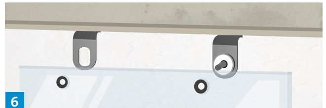
6 Insert the grommets into the holes in the glass panels, then align over the fittings.
